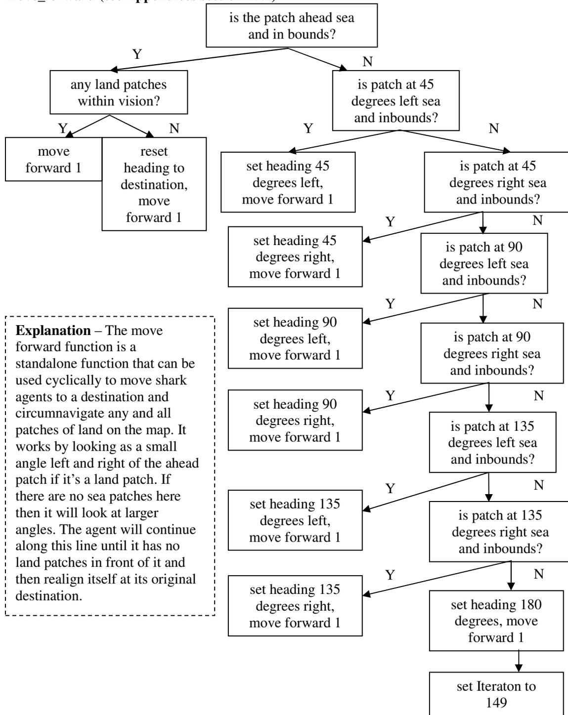
**Explanation** – The move forward function is a standalone function that can be used cyclically to move shark agents to a destination and circumnavigate any and all patches of land on the map. It works by looking at a small angle left and right of the ahead patch if it's a land patch. If there are no sea patches here then it will look at larger angles. The agent will continue along this line until it has no land patches in front of it and then realign itself at its original destination.
