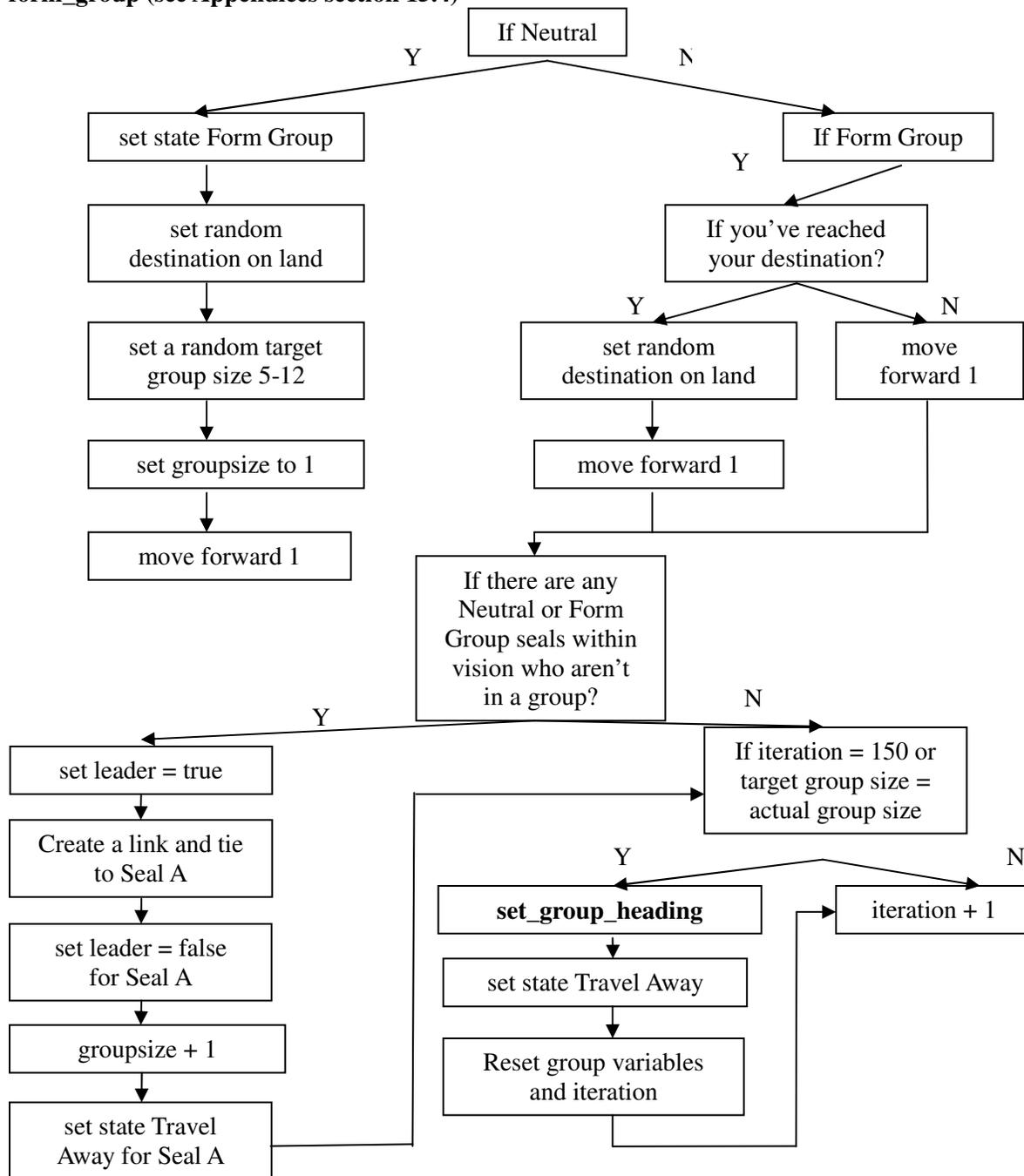
**Explanation** – The form\_group will set a target groupsize and cyclically choose destinations on land and travel to them until the seal in question has gathered enough seals to fit its target or until the iteration counter has reached 150. This is to break any looping for finding seals for a group that don't exist.
