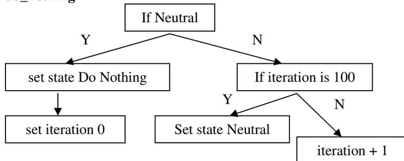
**Explanation** – The do\_nothing modules is a simple iteration that increments 100 times before returning to a Neutral state, imitating the seal doing nothing.
