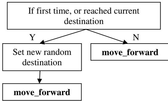
**Explanation** – The basic\_shark function is very simple and it is the only function called when the Intelligence? variable is false. It simply asks the shark agent if it has a new destination or has reached its current one. If so it sets a random new one at sea and calls **move\_forward**, otherwise it just calls **move\_forward**.
