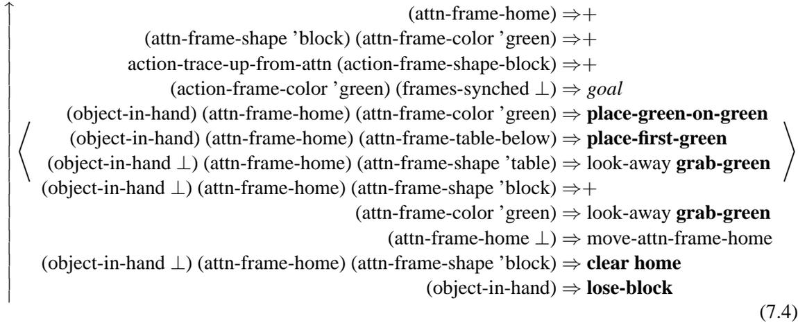
There is actually more information in the BRP than this notation represents. For one, each element is labeled with a name so that it is easier to see what that element does. For another, some elements actually have equivalent priority. Here is the list of the elements' names, with elements of shared priority on the same line. Notice that the elements are in the same order as they are above, this is simply another representation with different information.
