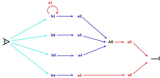
Figure 2-1: Behavior-oriented systems have multiple, semi-autonomous skill modules or *behaviors* ( $b_1 \dots$ ) which generate *actions* ( $a_1 \dots$ ) based on their own perception (derived from *sensing* indicated by the eye icon on the left). Actions which affect state outside their generating behavior, whether internal to the agent or external (indicated by the hand icon on the right), are generally subject to arbitration by an *action selection* (AS) system.
