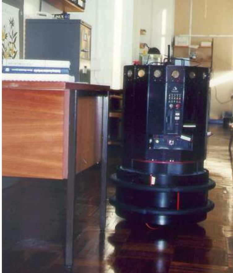
Figure 7-1: The Nomad 200 robot running in a laboratory at the University of Edinburgh. In this picture it has just encountered a desk — the surface is too low for the sonar sensors to detect when proximate, and the leg too dark for the infra-red sensors, so the robot had to learn about the desk with its bumpers.
