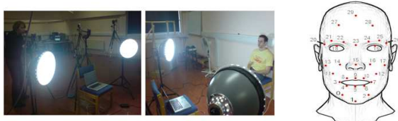
Figure 2: Motion Capture Set-Up: 30 retro-reflective markers are placed on a performer.
