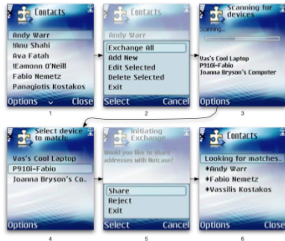
Figure 1. Using Bluetooth, a user needs to activate the exchange mechanism (photos 1 to 4). The second user is alerted to the request for exchange (photo 5). If the second user agrees, the phones carry out a two-way exchange of digests. Upon successful completion of the exchange, the phones present the common entries (photo 6).
