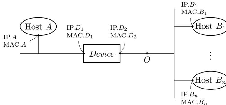
*Device* is a machine that can be configured as a bridge or as a router, IP.X and MAC.Y are, respectively, IP addresses and MAC addresses at several interfaces (where they might or might not be used) and *O* is a point where packets can be observed. We assume that the network mask 255.255.255.0 is in place for all the machines on the network. Please answer the following questions.
