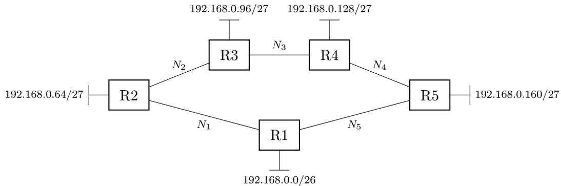
$R_1$ ,  $R_2$ ,  $R_3$ ,  $R_4$  and  $R_5$  are routers, each of which has three interfaces.  $N_1$ ,  $N_2$ ,  $N_3$ ,  $N_4$  and  $N_5$  are networks connecting the routers. Please answer the following questions:
